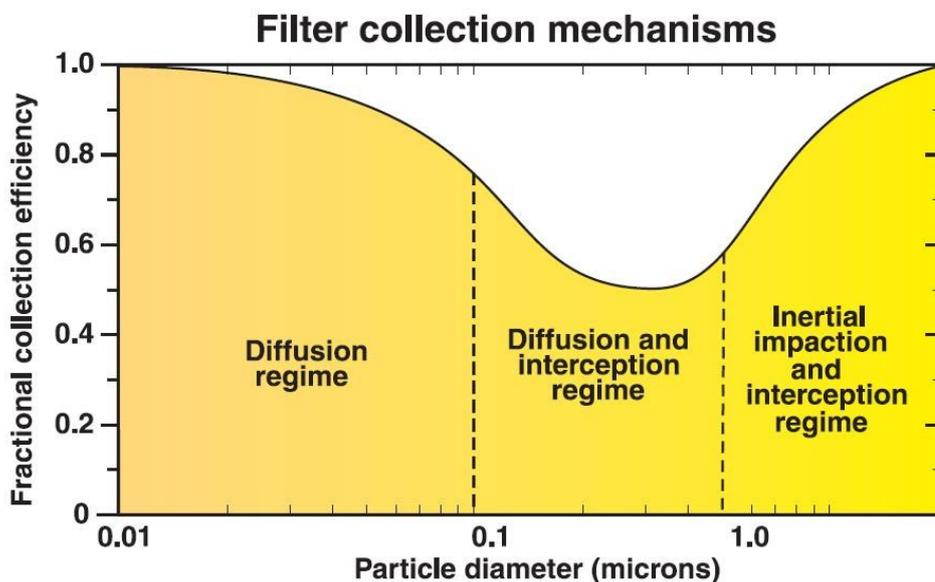
Figure 2 Fractional collection efficiency versus particle size for a mechanical filter.
