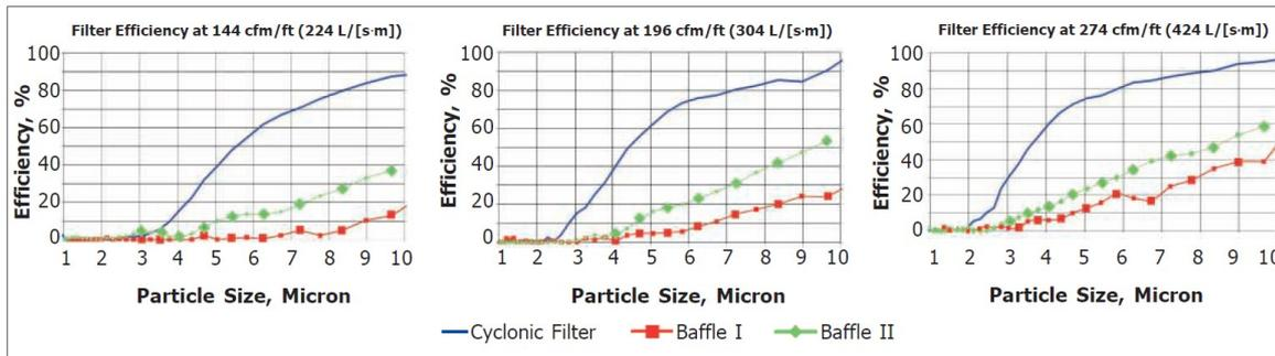
Figure 6 Grease filter efficiency as function of particle size for three exhaust airflows (Livchak et al., 2003)
