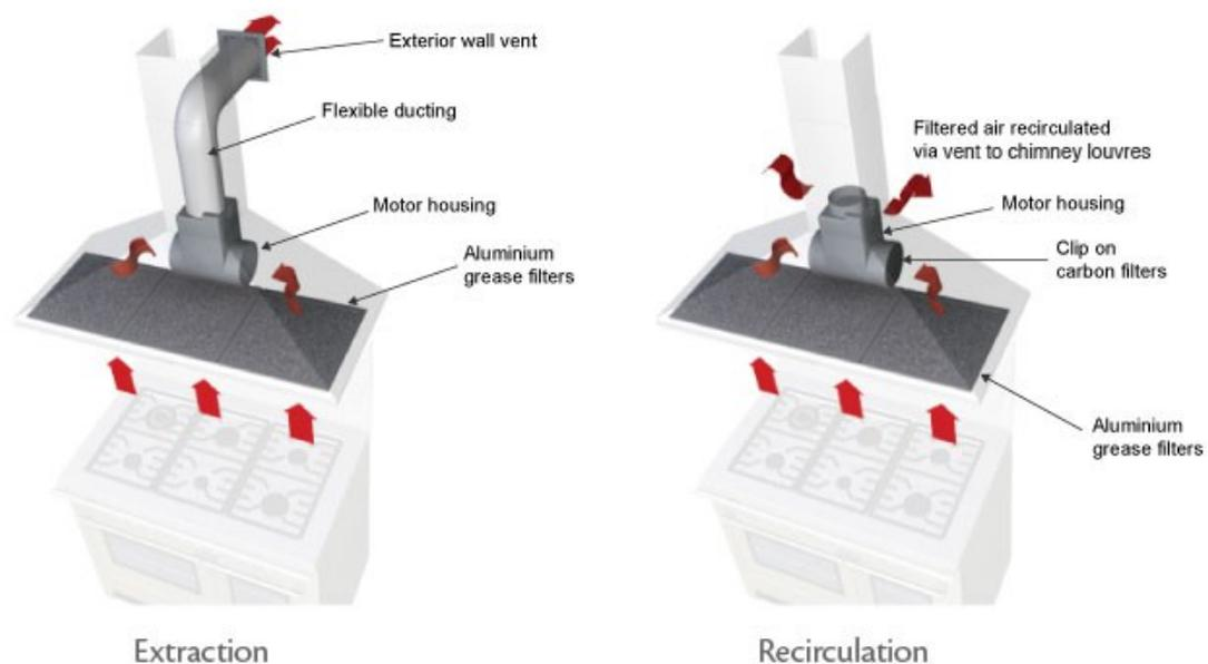
Figure 4 Schematic representation of typical extraction and recirculation cooker hoods (source: internet)
