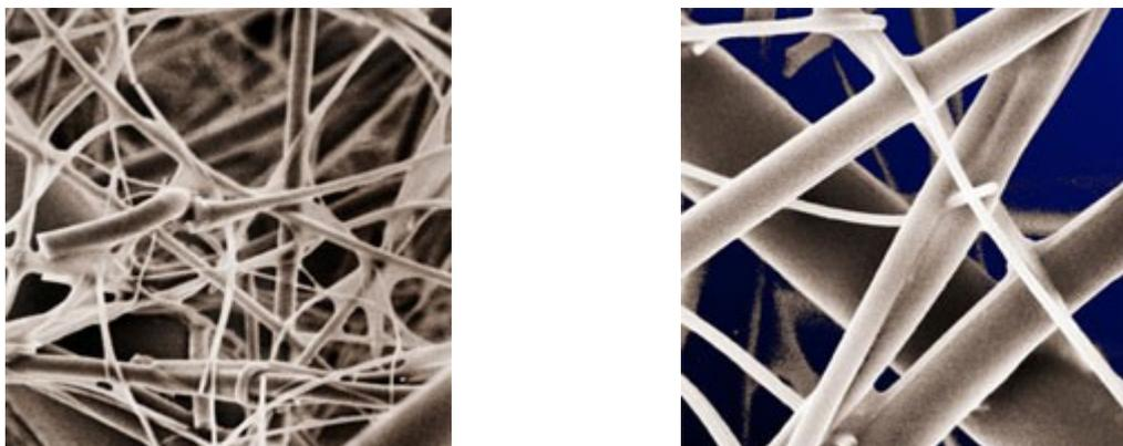
Figure 1 Electron microscope image of fibre media air filters
